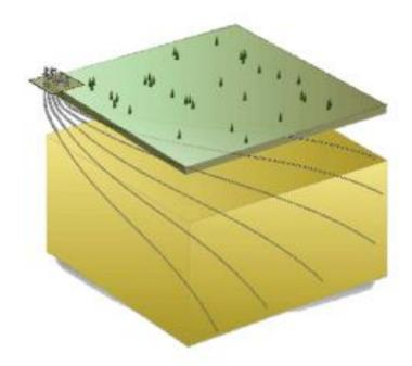
6 Horizontal wells (8 fracs/well) = 48 total fracs per section
